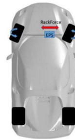
Fig. 41 Rack Force measured by EPS system
